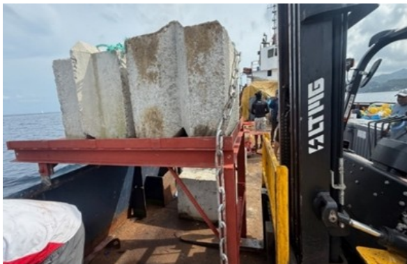
Figure 15: Forklift in position below the launch table preparing to release the FAD anchor blocks into the ocean.
